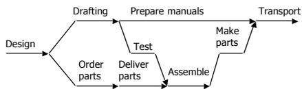
shows operations required to produce custom made machine
