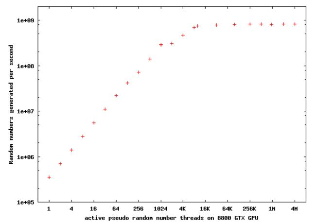
In test environment, with  $\geq$  8192 threads the 128 stream processors give peak performance. I.e.  $\geq$ 16 active threads per SP. Or  $\geq$ 512 threads per G80 8SP block. 20
