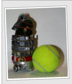
Constructed in-house, EMMA (EMbedded Mobile Agent) is based on the Khepera robot, but with improved CPU and vision.
